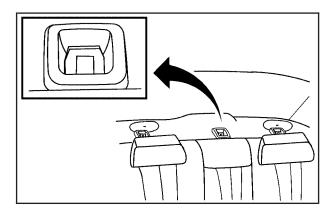
The top tether anchors are located behind the rear seat on the filler panel.
